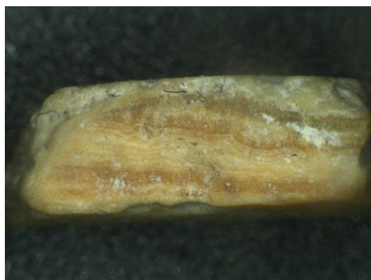
Fig. 5 Lamellar microstructure of sample B
